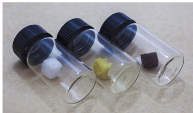
Figure 3. Photographs of the elastomeric foam before (white), after the ZnSe loading (yellow) and after the removal of \text{Pb}^{2+} ions from water (dark brown).
